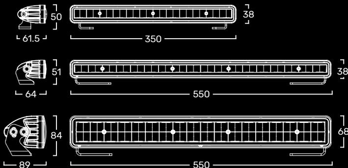
Dimensions are measured in mm with 2 'L' mounting brackets.
